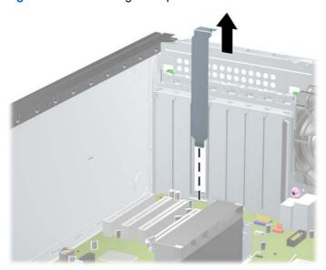
Figure 5-10 Removing an Expansion Slot Cover
